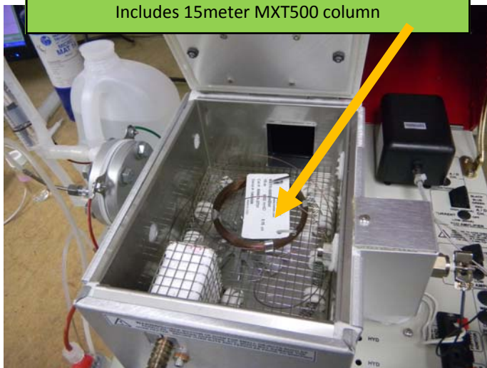
The temperature programmable column oven heats from ambient to 400C.
