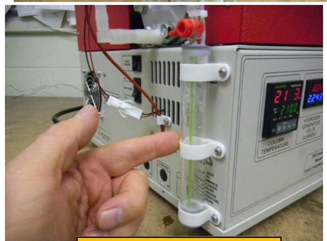
The water separator is mounted on the left front of the GC
